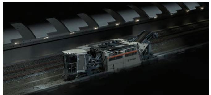
ALL IMAGES: The 260 SX(i) cross application miner can cut, crush and discharge the material in a single operation to a width of 2.75 m and a depth of up to 650 mm.
